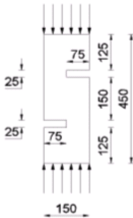
Fig.1 Push-off specimen without side face reinforcement
